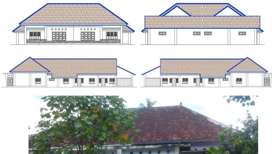
Figure 9. Roof shape of second house.
