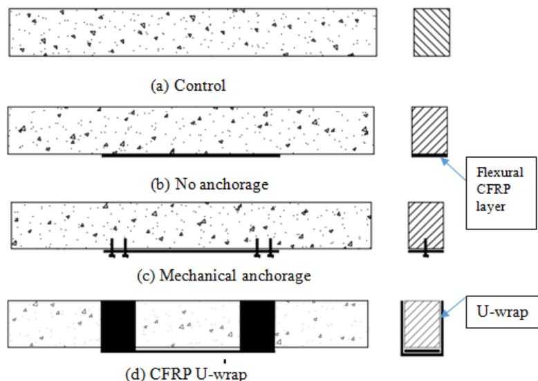
Fig.4. CFRP and anchorage schemes
