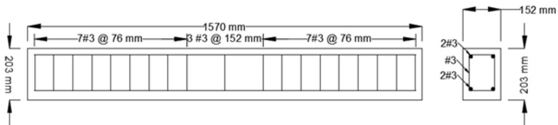
Fig. 3. Test beam details
