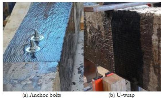
**Fig.6. Mechanical and U-wrap anchor**
