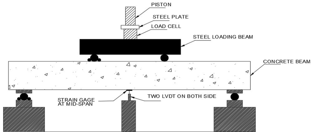
**Fig.7. Test schematic**
