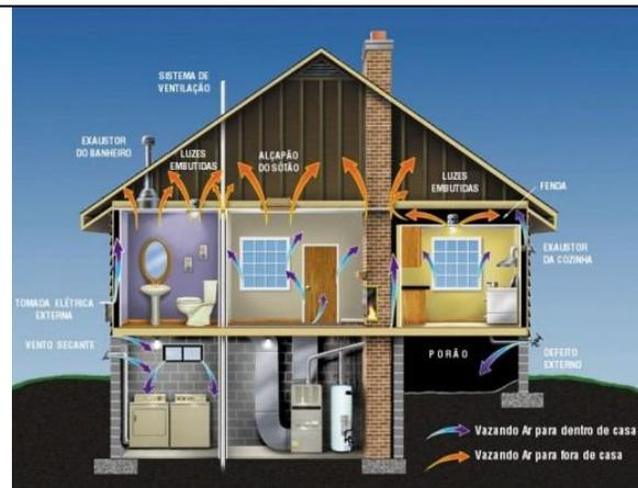
**Figure 05: Scheme of possible forms of Infiltration in a Residence. Source: Ecopore of Brazil**
