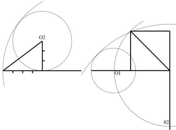
**Fig. 1: Left: Drawing Method of a pre-Islamic Arch in Iran (Ghyka(1977:23). Right: drawing Method of *Panj-o-haft* arch (Pirnia 2008: 103). Safavid arch has less Thrust (Drawn by author)**
