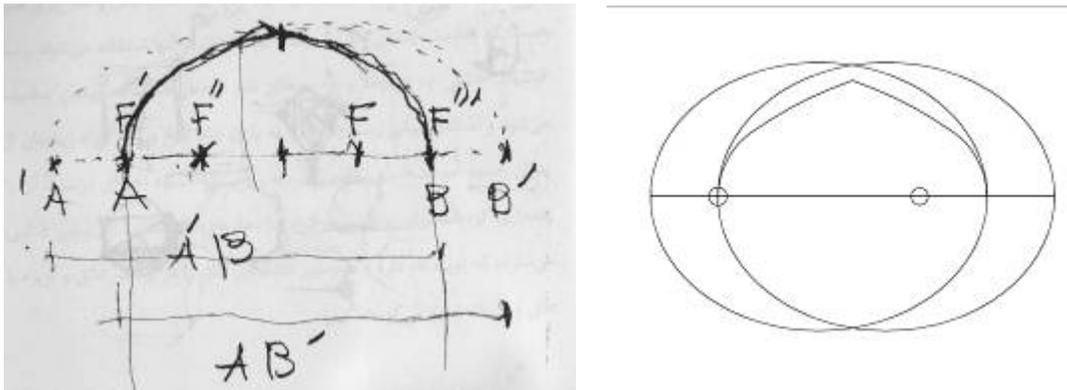
**Fig. 2: Left: A drawing by Pirnia, who Considered the Pointed Arch as the Intersection of two Ellipses (Pirnia 2008: 103). Right: Author's drawing shows the Difference between arch Geometry and Pirnia's Method**
