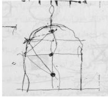
**Fig. 3: Pirnia's drawing Of the Tool *Shāhang-O Hanjār* for Constructing Elliptical Domes (Pirnia 2008:103).**
