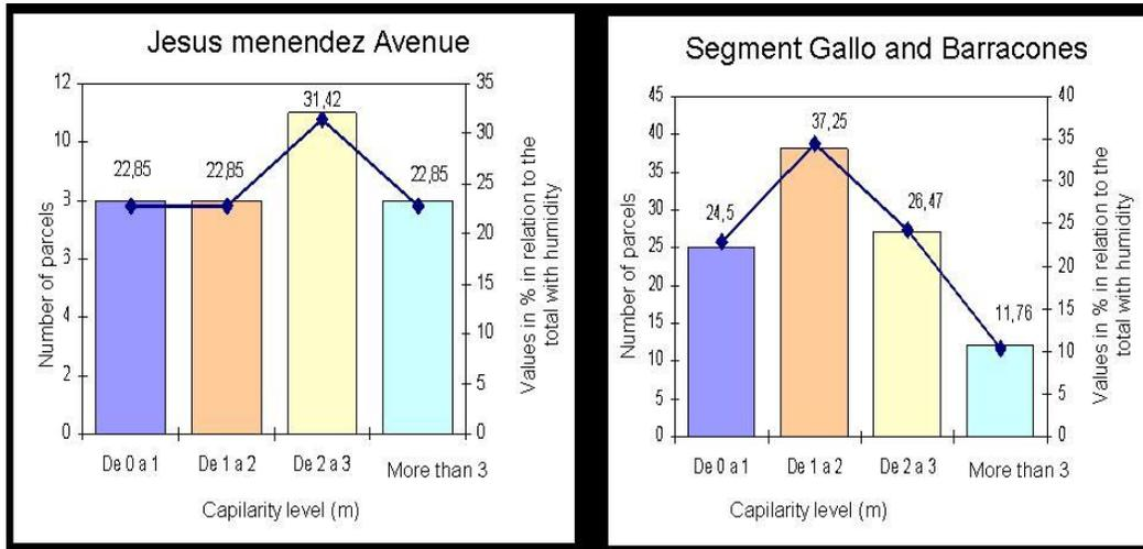
**Figure 2: Results of Capillary Height Measurements in the Studied Sections in the Lower Part of the Historic center of Santiago de Cuba**
